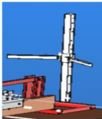
Figure 4 – General view of the impact resistance test device
